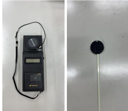
Figure 3. Illuminometer (left) and Direct Sunlight Block (right)
